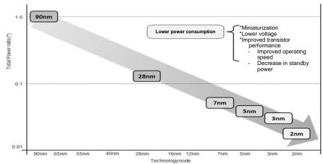
\* The vertical axis is the relative ratio of each technology with respect to the 90nm Total Power (sum of Dynamic and Leakage components).
